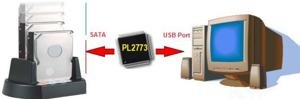
The PL2773 JBOD solution also allows you to add another unique standalone feature called AutoMirror. This automirror solution does not require any PC connection and works by simply pressing the Backup Button for 3 seconds which will automatically mirror the entire SATA1 Source HDD sector by sector (including boot sector, partition table and file system format) to the SATA2 Destination HDD. (NOTE: All original data in the Destination HDD will be destroyed.)
