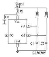
C0: decoupling capacitor 0.1uF~2.2uF (recommended)
