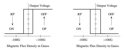
Fig 2. Magnetic Hysteresis Characteristics
