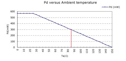
Fig 4. Pd vs ambient temperature
