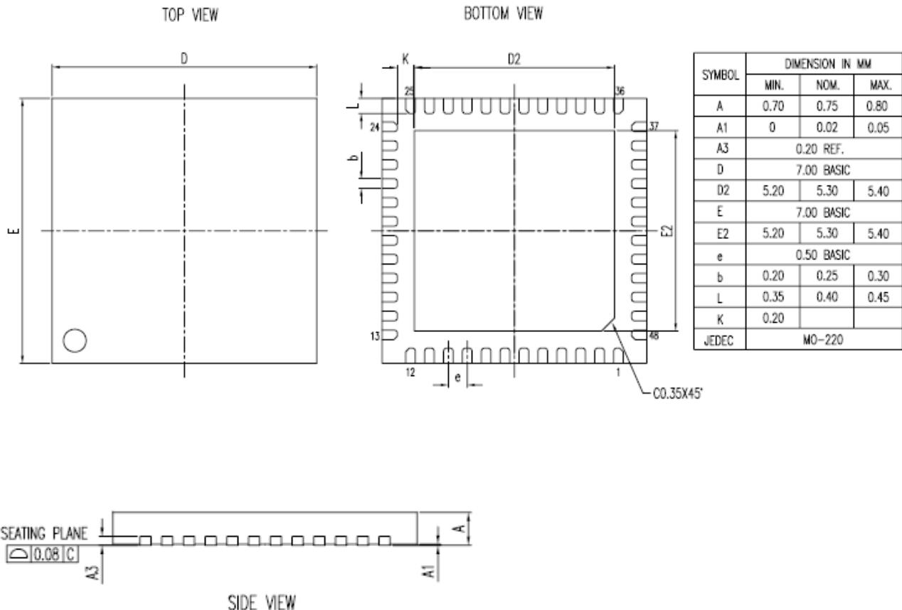
Figure 10-1: PL2523 Outline Diagram (QFN48 7x7mm)
