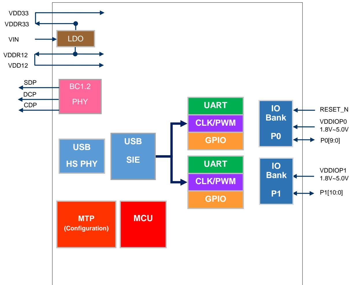
Figure 4-1: PL2523 Block Diagram
