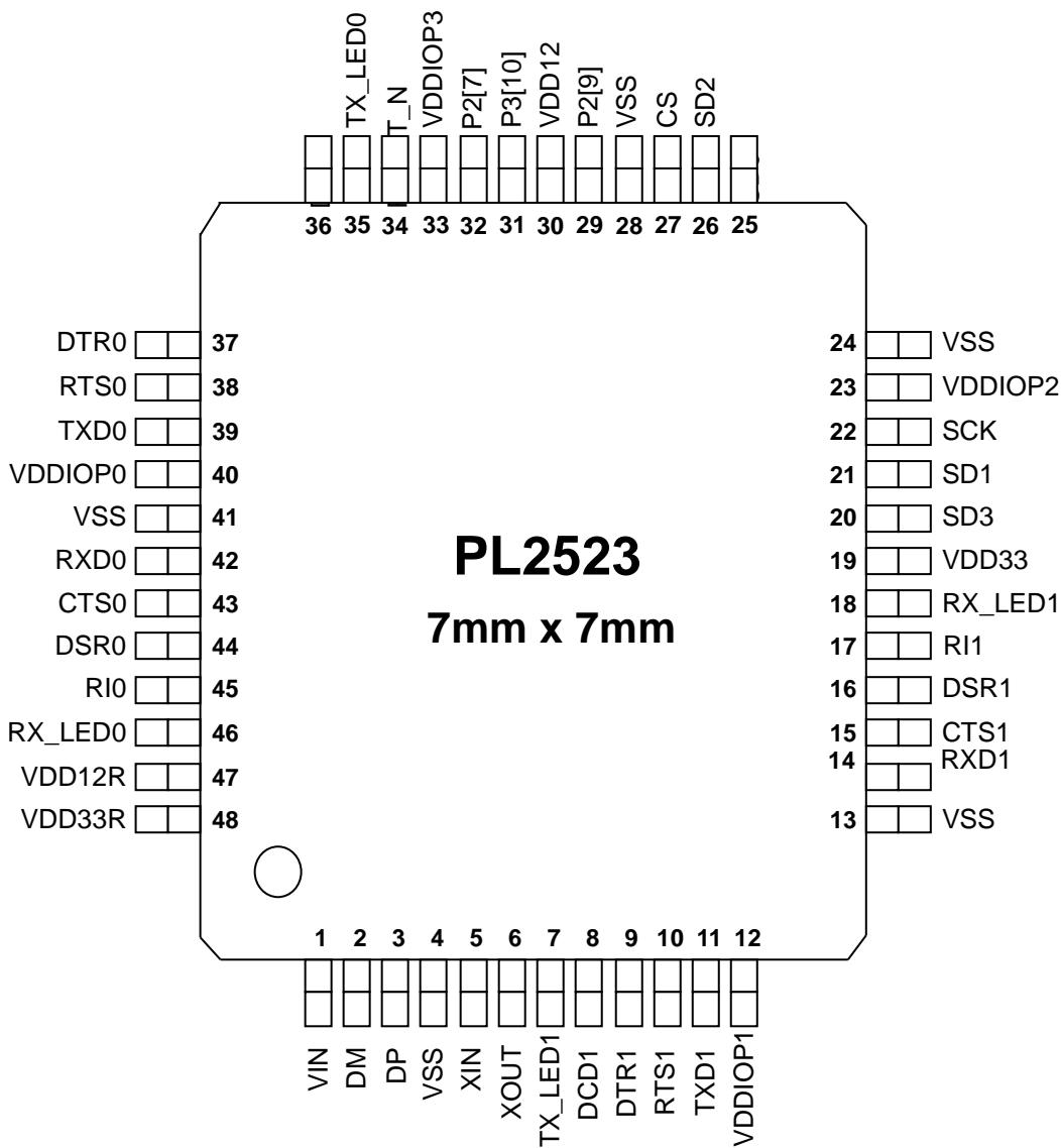
**Figure 7-1: PL2523 Pin Diagram**
