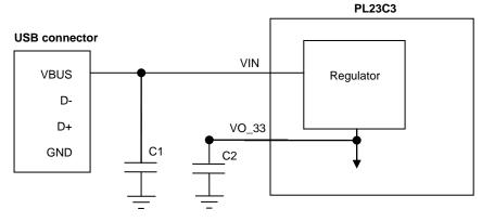
Figure 10-1 USB Bus Powered Design Example
