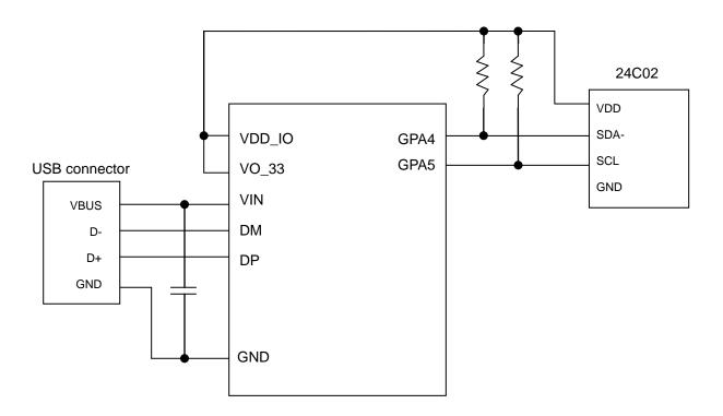
Figure 10-6 External I2C EEPROM Design Example
