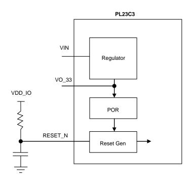
Figure 10-3a Chip Reset Control Application
