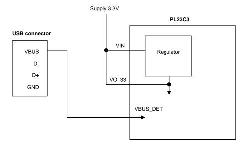
Figure 10-2b USB Self Powered Design Example 2
