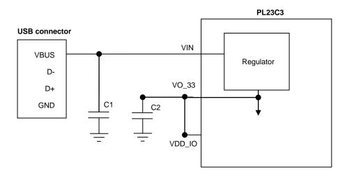
Figure 10-4a IO Power Supply
