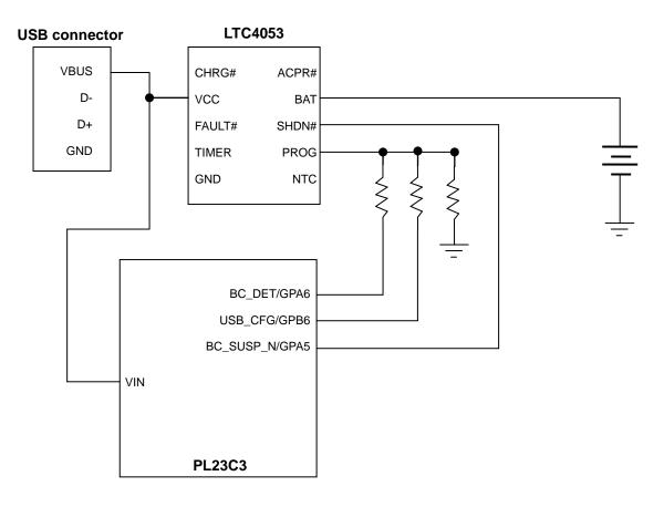
Figure 10-5a Battery Charging Design Example #1
