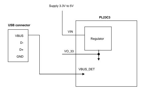
Figure 10-2a USB Self Powered Design Example 1
