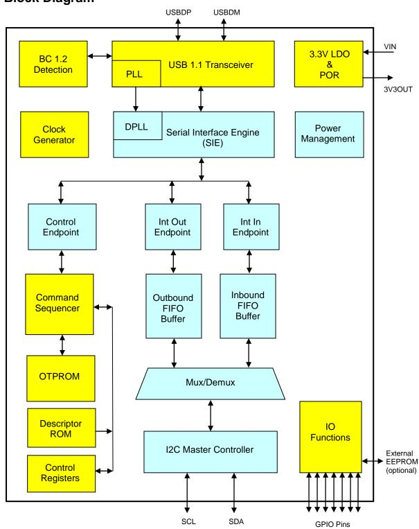
Figure 4-1 PL23C3 Block Diagram
