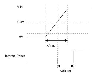
Figure 10-3b Chip Power Reset Timing Diagram
