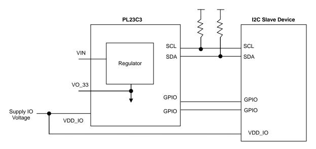
Figure 10-4b VDD IO Voltage Supply
