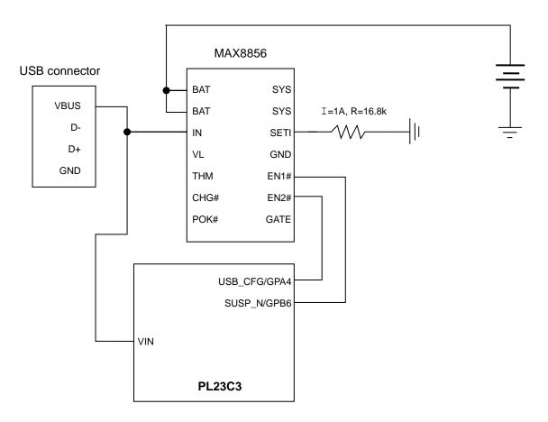
Figure 10-5b Battery Charging Design Example #2
