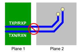
Avoid signal reflection – Route USB/SATA differential signal pair should not change layer by vias [see below Figure no. 3], and avoid branch trace by via [see below Figure no. 2]. These can reduce signal reflection and impedance change. If it is necessary to turn 90° [see Figure below no. 1], it is better to use two 45° turn or an arc instead of making a single 90° turn. This can reduce reflection on the signal by minimizing impedance discontinuities.
