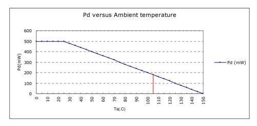
Fig 1 Pd vs ambient temperature
