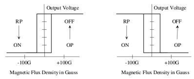
Fig 3. Magnetic Hysteresis Characteristics
