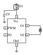
C0: decoupling capacitor 1nF ~ 0.01uF
