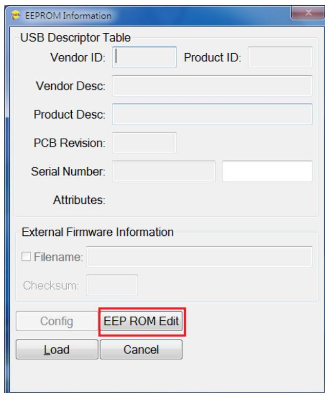
2. Make sure the device drive is detected before you can write the configuration. Click the Load EEP button first to load the PL2775 RAID SDT configuration file.
