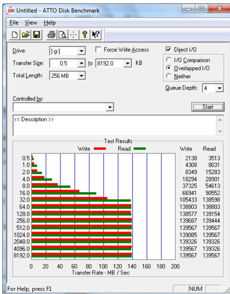
**RAID1 Mode HDD Performance (USB3 Host Under PCIe GEN2 Interface)**
