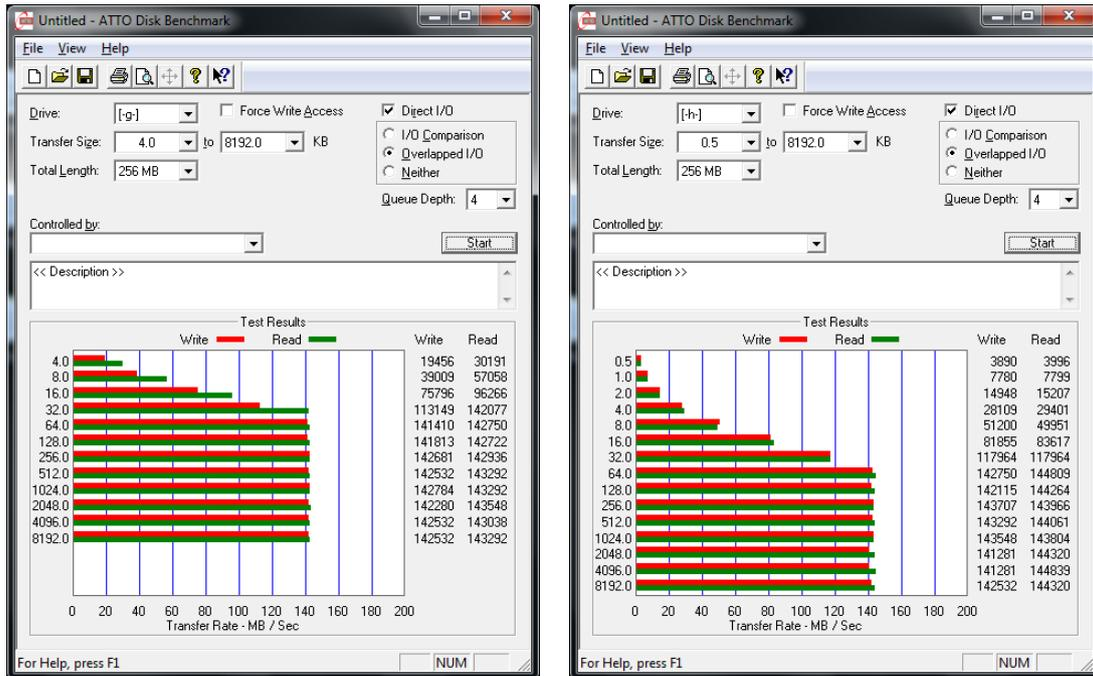
**JBOD HDD Performance (USB3 Host Under PCIe GEN2 Interface)**
