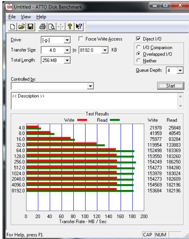
**RAID0 Mode HDD Performance (USB3 Host Under PCIe GEN2 Interface)**
